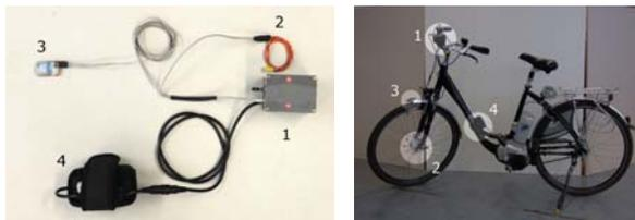
German NCS data acquisition system. (1) box with cameras and LEDs; (2) speed sensor; (3) GPS sensor; (4) battery package.
