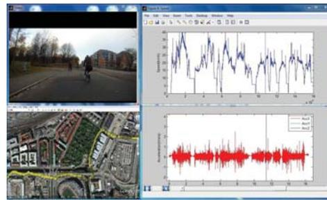
Analysis tool view out of the Swedish NCS. Top left: front view (video); bottom left: map view (GPS); top right: speed (speed sensor); bottom right: acceleration (IMU).
